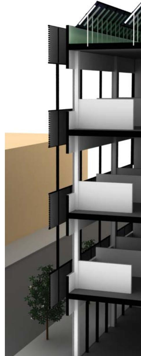
b) Evacuated tube solar collectors: we incorporated evacuated tubes on the Southern façade in order to heat water for plumbing uses. Along our façade we located several modules which contain in total 405 tubes that would produce a total of 5491 Btu/sf/yr and 19.7% of the energy needed. The information for our calculations was taken from the solar hot water system website
