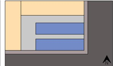
4. Building footprint covers most of site but offset from surrounding buildings. The building is split into two sections around a central atrium space. This allows for more daylight to enter into the building (from the center and all facades.) Thermal gain/loss is from all facades.
