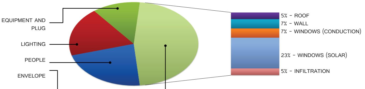
COOLING LOAD COMPONENTS FOR A TYPICAL 10,000 SF OFFICE BUILDING
