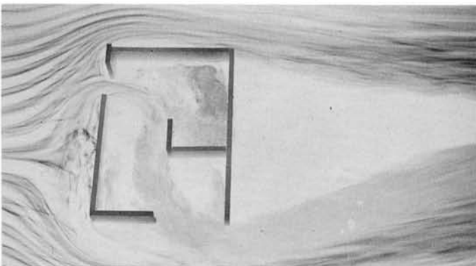
Figure 9: Improper partitioning of a space can inhibit windflow.
